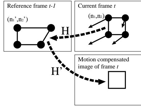
Figure 4. Motion compensation procedure for a block.
