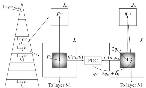
Figure 2. Block matching using a hierarchical coarse-to-fine approach.
