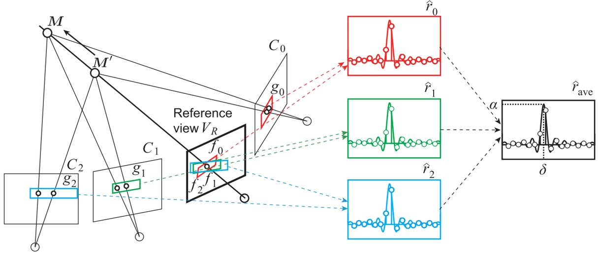
**Fig. 1** Depth estimation using POC-based window matching: The initial 3D point  $M'$  is projected onto stereo image pairs. POC functions  $\hat{r}_i$  are calculated from the matching windows which are extracted from each stereo image pair. The average POC function  $\hat{r}_{ave}$  is calculated from the POC functions. The true 3D point  $M$  is obtained by estimating the peak position of  $\hat{r}_{ave}$ .
