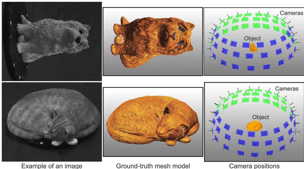
**Fig. 3** Example of an image, a ground-truth mesh model, and camera positions in our MVS dataset (Upper: dog, Lower: cat).
