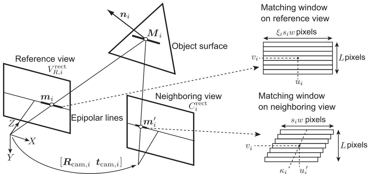
**Fig. 2** Matching windows for POC-based window matching with geometric correction for MVS: Assuming that each local region of the object is approximated by a 3D plane, the image transformation between the matching windows can be approximated by scaling and skewing. Local scaling can be reduced by scaling the size of window on the reference view. Local skew can be reduced by skewing the matching window on the neighboring view.
