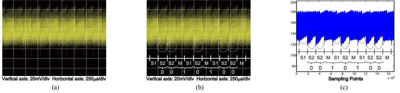
Fig. 5. Power waveforms of CIOS processor using an embedded multiplier: (a) random value input, (b)  $N - 1$  value input, (c)  $N - 1$  value input and filtering.
