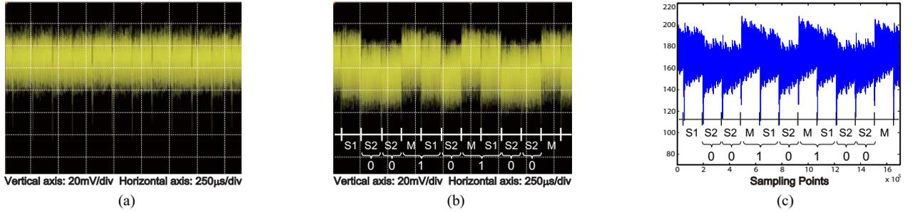
Fig. 6. Power waveforms of FIOS processor using an embedded multiplier: (a) random value input, (b)  $N - 1$  value input, (c)  $N - 1$  value input and filtering.
