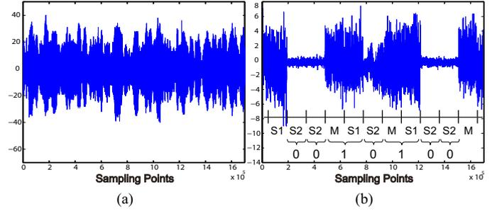
Fig. 9. SPA using  $X$  and  $-X$  value inputs (CIOS): (a) difference waveform, (b) filtered difference waveform.
