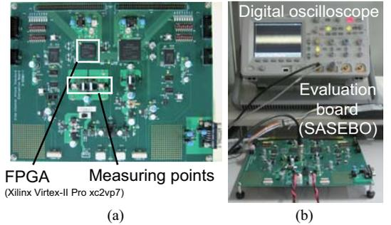
Fig. 4. (a) Evaluation board (SASEBO), (b) Experimental environment.
