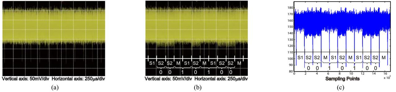
Fig. 7. Power waveforms of CIOS processor using a custom array multiplier with booth encoder: (a) random value input, (b)  $N - 1$  value input, (c)  $N - 1$  value input and filtering.
