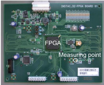
**Fig. 14** Evaluation board (INSTAC-32).
