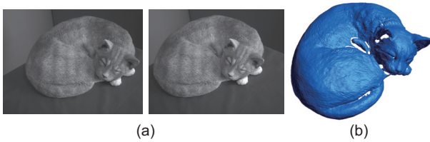
Fig. 2. Performance evaluation using a fixed stereo camera: (a) stereo images (1,280×960 pixels) and (b) ground truth 3D model measured with KONICA MINOLTA VIVID.
